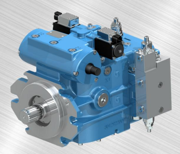
The HD1 Series variable piston pumps for closed loop circuits are axial pistons pumps with swash plate design and through drive shaft on option. These pumps have been specifically designed for use in closed circuit hydrostatic transmissions.
